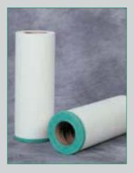
At the heart of the RMF Off-line and By-pass filter units is the unique microfilter element. This filter works according to the radial through-flow principle. As it has a filter fineness of 0.5 micron, it is able to remove the smallest of contamination particles (silt) from the oil.
