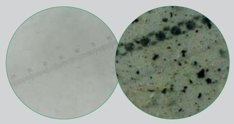
Mainstream filters are incapable of removing the smallest particles, smaller than 2 micron (better known as silt). Fluctuations in the supply and the resulting changing conditions mean that these filters cannot carry out fine filtration; most of the silt remains in the system and affects the chemical composition of the oil.
